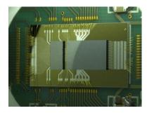
DEPFET Current Digitiser (DCD) 256 channels, 10-bit, 10 MHz ADCs, 65 400 MHz Links
