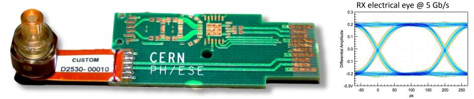
TOSA and commercial Laser Driver on VTRx PCB •
