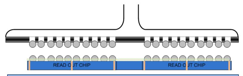
Solder mass transfer is very efficient process to attach the solder spheres to wafer
