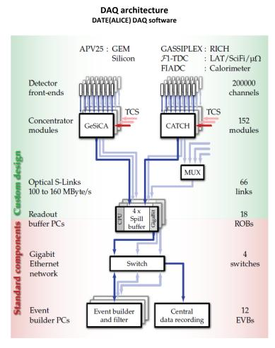
Maximum trigger rate: 30kHz
