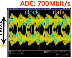
Performance limited by no-impedance on XILINX-evaluation board Eye diagram is well open
